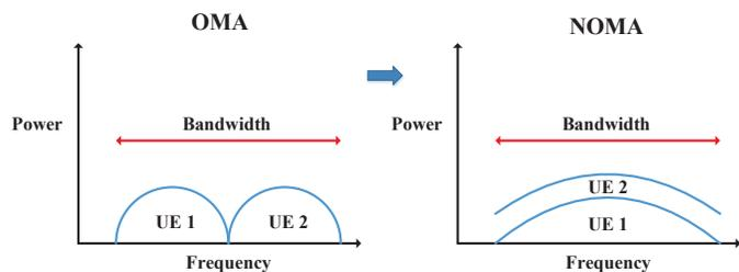
Fig. 2: Simple comparison between OMA and NOMA with  $K=2$ .
