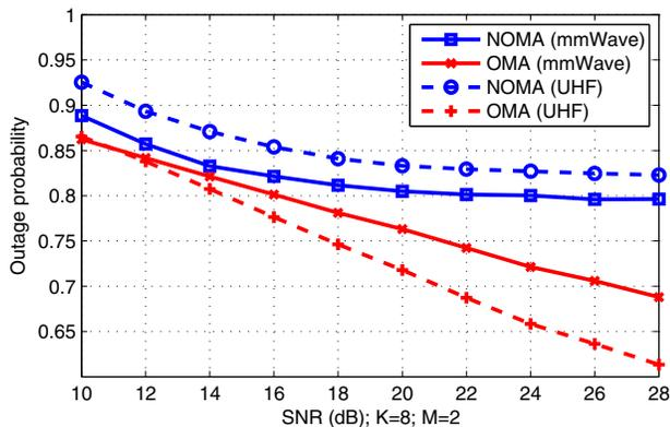
Fig. 7: Outage probability versus operating SNR.
