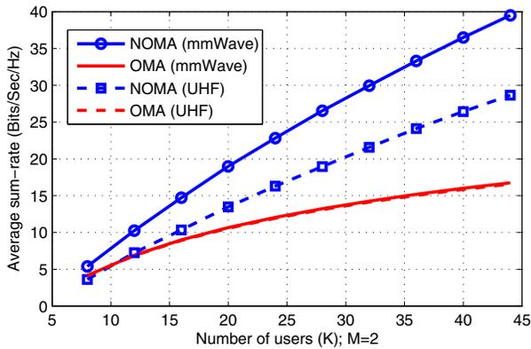
Fig. 3: Spectral efficiency versus number of users.
