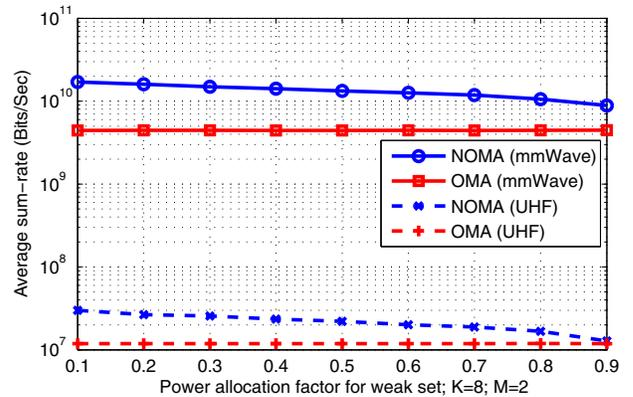
Fig. 5: Average sum-rate versus the power allocation factor,  $\beta_2$ .
