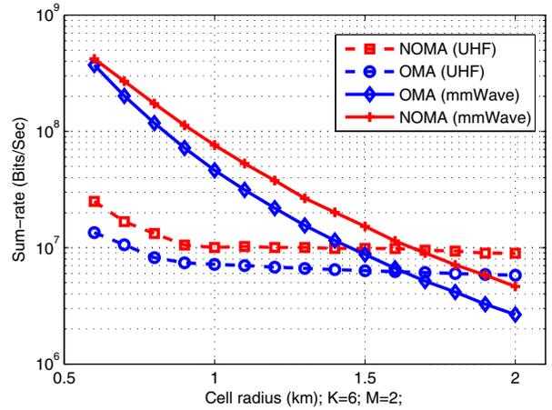
Fig. 4: Average sum-rate versus cell radius.
