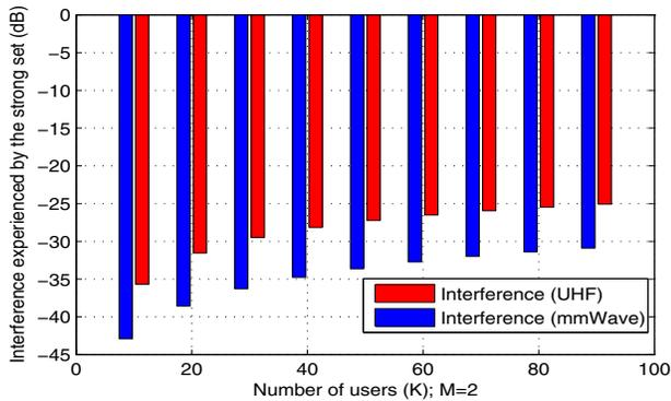
Fig. 6: Interference levels experienced by members of the strong set versus total number of users in the cell.
