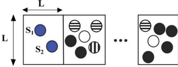
Fig. 1. Realization of a strip-shaped network topology with randomly placed nodes;  $N = 6$
