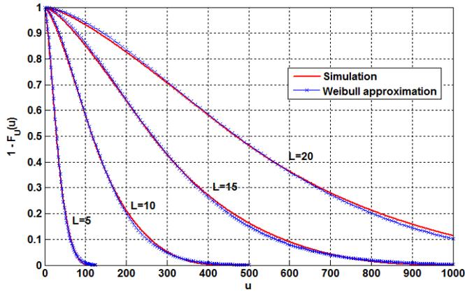
Fig. 4. Tail probabilities of analytical model and the Weibull approximation for different values of  $L$ .
