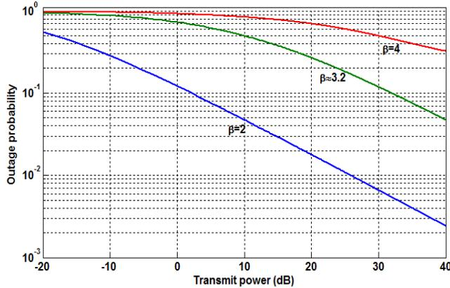
Fig. 5. Effects of transmit power on the outage probability for different path loss exponents  $\beta$ .  $L = 10$ ,  $\tau = 0.001$ .
