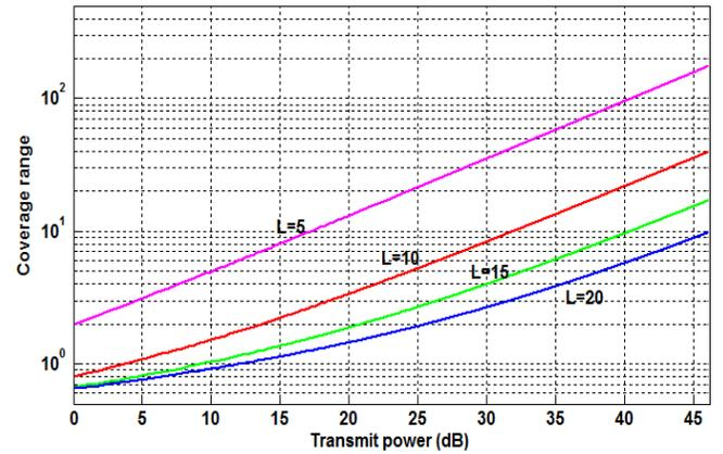
Fig. 6. Effects of transmit power on coverage range for different region lengths  $L$ .  $\beta \approx 3.2$ ,  $QoS = 0.9$ ,  $\tau = 0.001$ .
