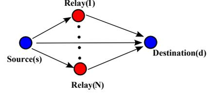
Fig. 2: Simplistic model of cooperative communication through relays
