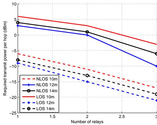
Fig. 4: Range extension experiment to determine the hop power required to maintain a BER of  $10^{-4}$  at the destination.
