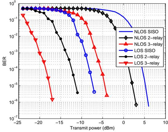
Fig. 3: Comparison of BERs between multi-hop SISO and CT topologies at a fixed coverage distance of 12m.
