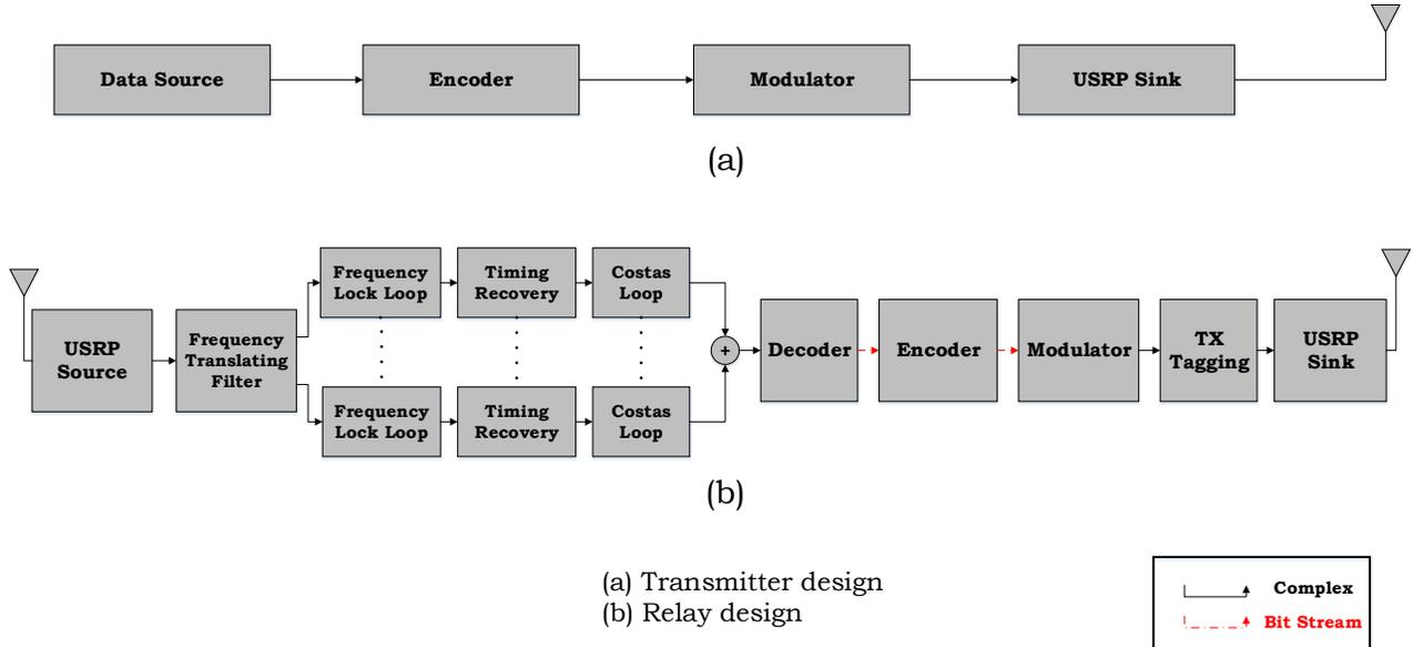
Fig. 2: Transceiver Design
