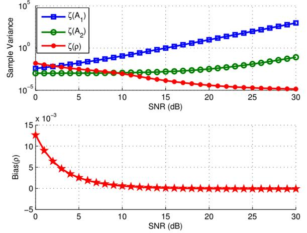
Fig. 1. Sample variance of error for different parameters and bias of CFO estimator;  $g=1000$
