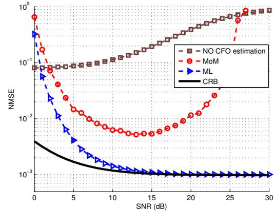
Fig. 3. NMSE plot for different SNR estimators;  $M = 8$ ,  $g = 1000$ .
