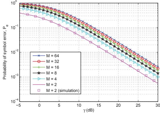
Fig. 1. The probability of symbol error against SNR for different orders of FSK,  $M$ ;  $K = 3$ .
