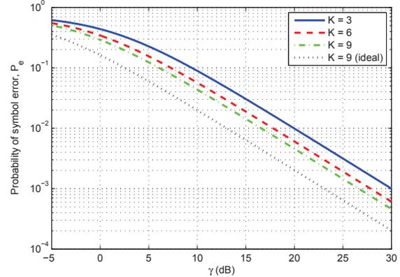
Fig. 2. The probability of symbol error against different number of transmitting nodes,  $K$ ;  $M = 4$ .
