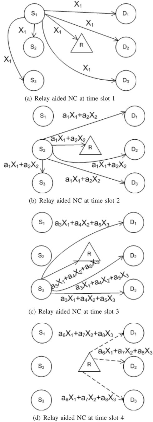
Fig. 2. Transmission pattern of relay-aided-network-coded (RANC) D2D
