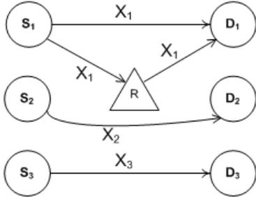
Fig. 1. Relay aided 3-D2D pair network
