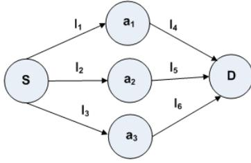
Fig. 2: Two-hop D2D network
