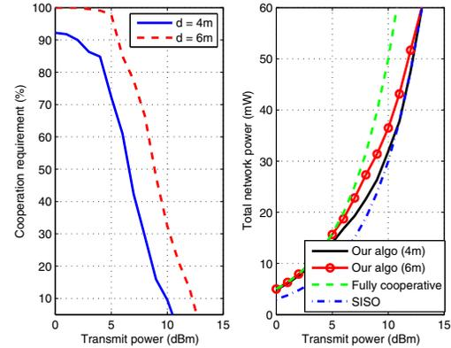
Fig. 10: Left: Percentage of cooperative transmissions against node transmit power. Right: Comparison of network energy efficiency for fully cooperative and SISO networks, with our proposed algorithm.
