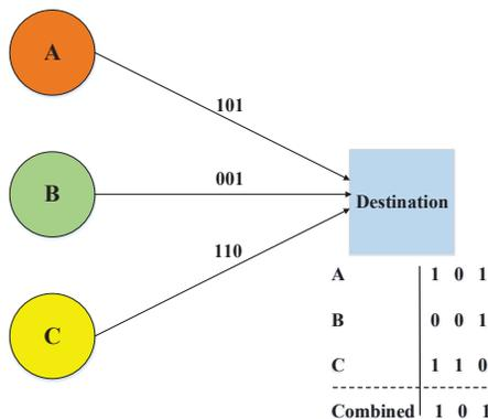
Fig. 4: Post-detection combining.
