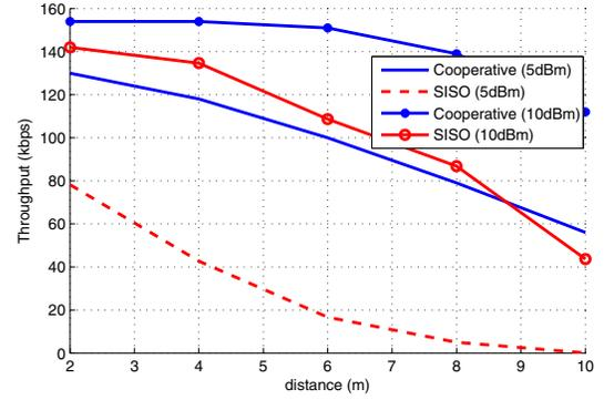
Fig. 9: Throughput versus S-D distance for SISO transmissions and CT.
