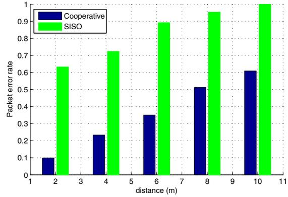
Fig. 8: PER for the two network topologies versus S-D distance at transmit power = 5dBm.
