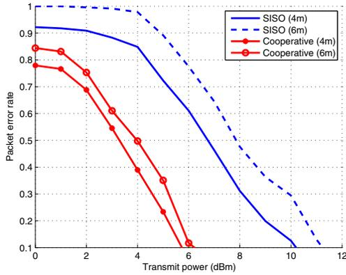
Fig. 6: Comparison between SISO transmissions and CT for S-D distances of 4m and 6m, in terms of PER for varying transmit power.
