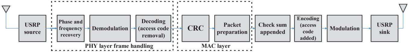
Fig. 3: Transceiver design.
