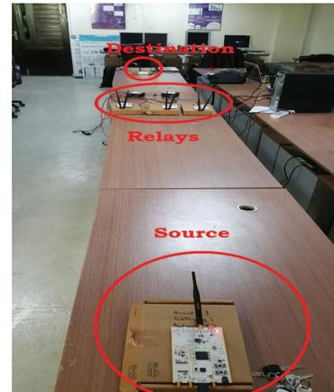
Fig. 5: The experimental setup.
