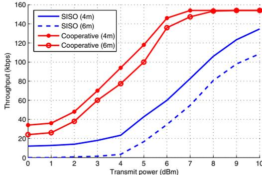
Fig. 7: Throughput versus transmit power for SISO and cooperative links.
