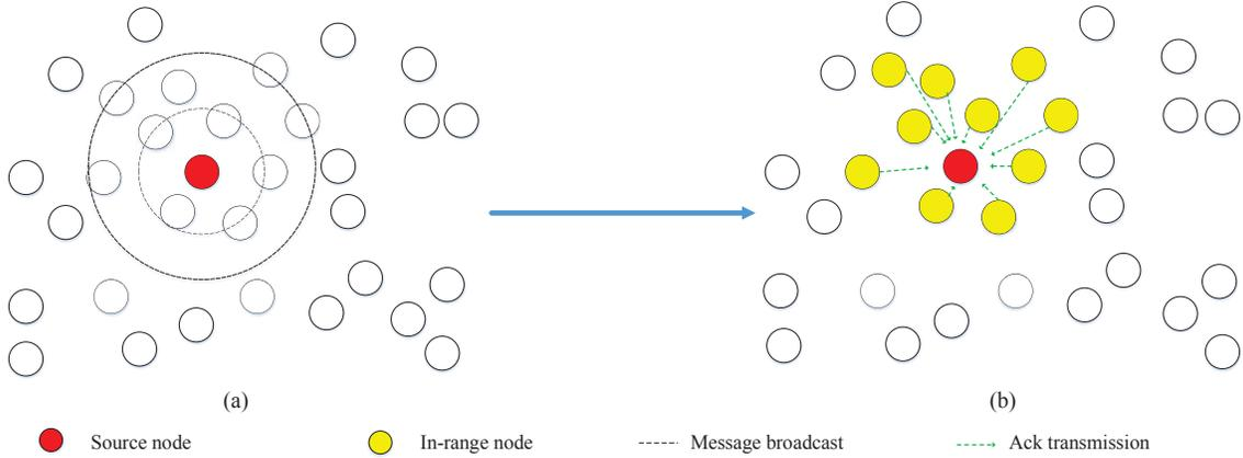
Fig. 1: (a): The source broadcasts its message, (b): The nodes that receive this message, transmit ACKs back to the source.
