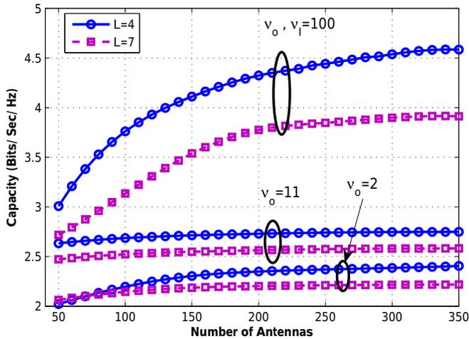
Fig. 2: Downlink rates for different shadowing intensities with RZF precoder,  $K = 10$
