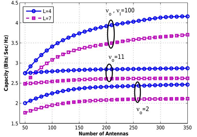
Fig. 3: Downlink rates for different shadowing intensities with BF precoder,  $K = 10$
