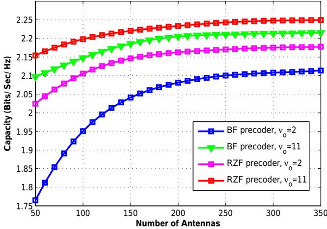
Fig. 1: Downlink rates for different shadowing intensities with RZF, BF precoders,  $L = 7$ ,  $K = 10$
