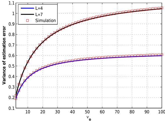
Fig. 4: Estimation error variance for different shape parameters,  $K = 10$ ,  $M = 50$ .
