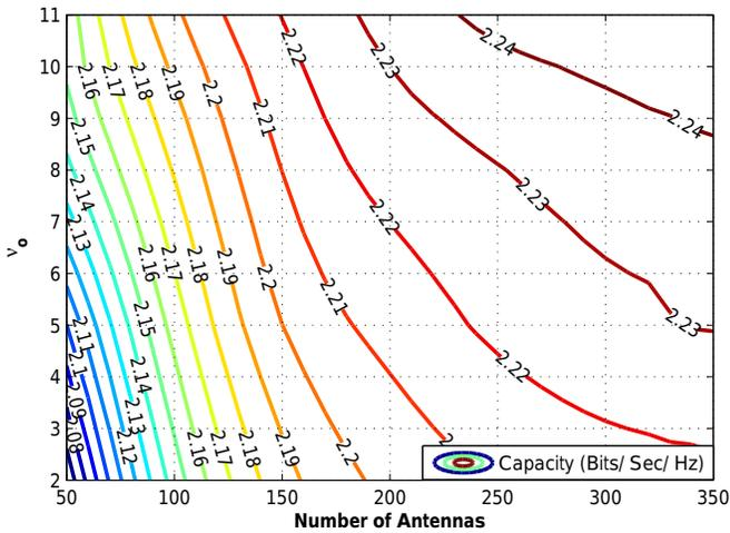
Fig. 5: Downlink rates for RZF precoder as a function of number of antennas and  $v_0$ ,  $K = 10$
