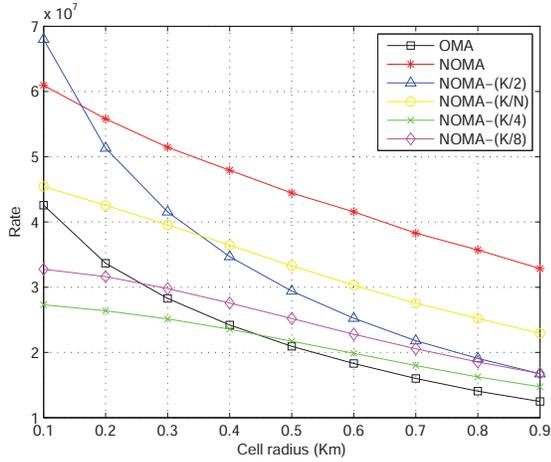
Fig. 5. Impact of cell radius on SBD scheme ( $N=2$ ,  $K=40$ ).
