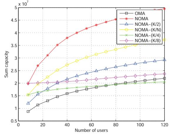
Fig. 3. Comparison of sum capacity of OMA, NOMA and proposed SBD scheme.
