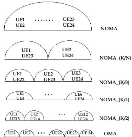
Fig. 2. OFDMA vs. NOMA and proposed SBD scheme,  $K=24$  for this particular example.
