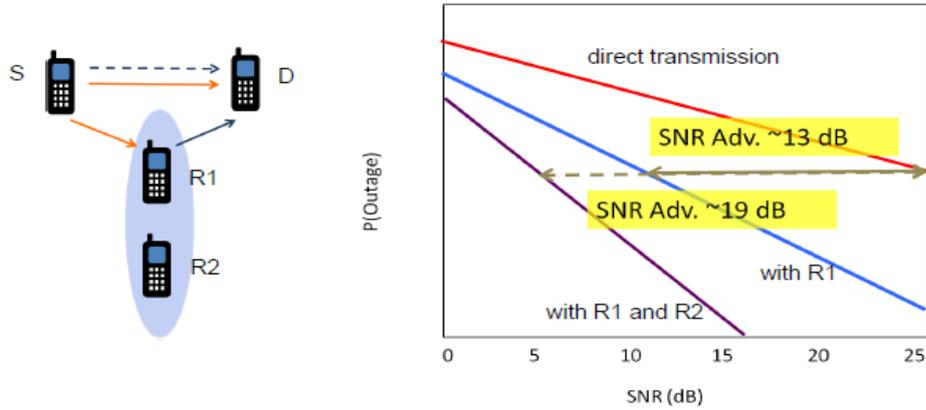
Figure 2.1: (Left): Cooperative and direct transmission topologies. (Right): Probability of outage for a given SNR for these topologies. [1]
