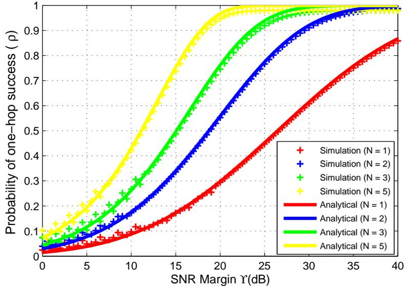
Figure 5.7: Simulation versus analytical results for  $L = 5$ ,  $\beta = 2$ ,  $\sigma = 6dB$
