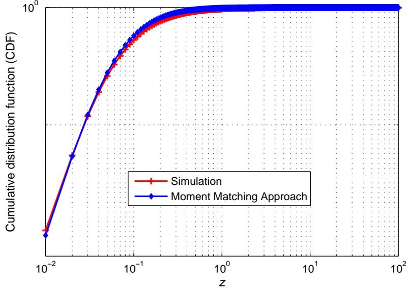
Figure 5.6: CDF comparison of theoretical and simulation approaches,  $\beta = 2$ ,  $L = 2$ ,  $\mu_\phi = 0dB$ ,  $\sigma_\phi = 6dB$ ,
