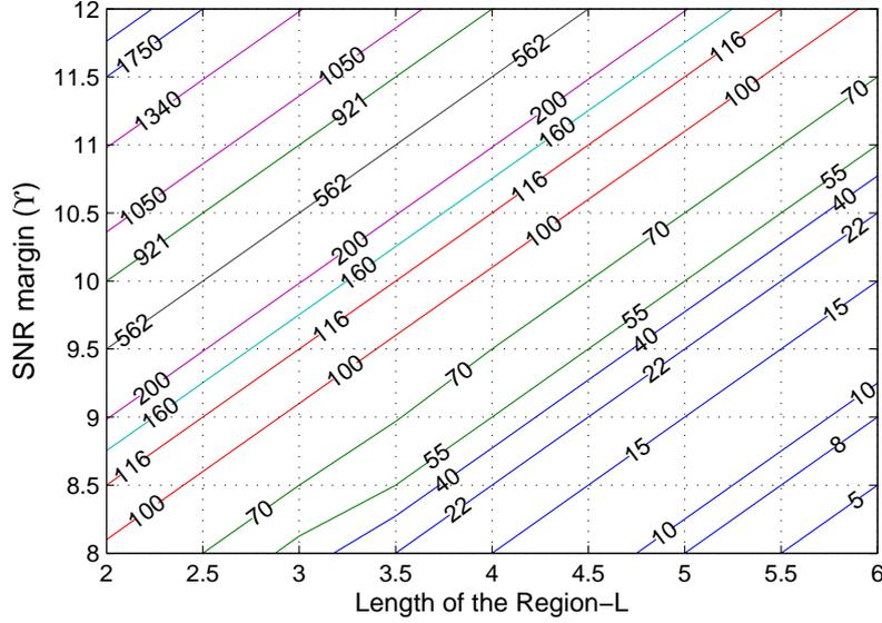
Figure 5.11: Coverage range for the extended strip network for  $N = 2$ ,  $\sigma = 6dB$  and  $\eta = 0.85$
