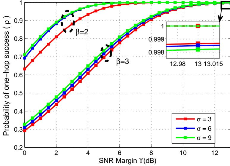
Figure 5.8: Varying standard deviation for different values of path loss exponent  $N = 3, L = 2$
