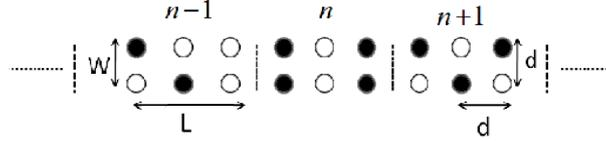
Figure 3.1: A 2D grid network with  $L = 3, W = 2; M = 6$
