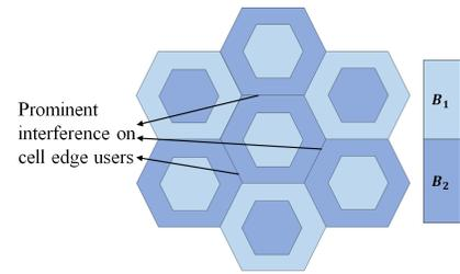
Figure 2: 2-RFA in a multi-cell scenario. The cell area is divided into two regions with frequency bands  $B_1$  and  $B_2$ .
