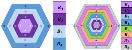
Figure 3: Frequency allocation in a single cell (4-RFA and 8-RFA).
