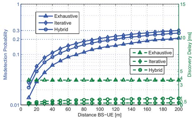
Fig. 3. Distance vs misdetection probability and discovery delay.
