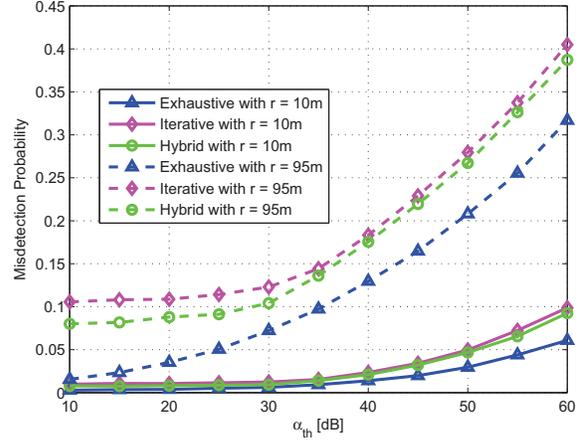
Fig. 1. Misdetection probability for the three algorithms at  $r = 10\text{m}$  and  $r = 95\text{m}$ .
