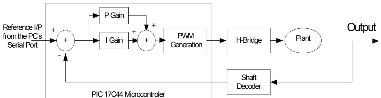
Fig. 3. Control scheme for the 2DOF Platform
