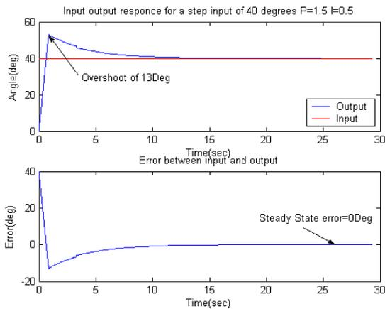
**Fig. 14. Input output plot for a step input and PI gains**
