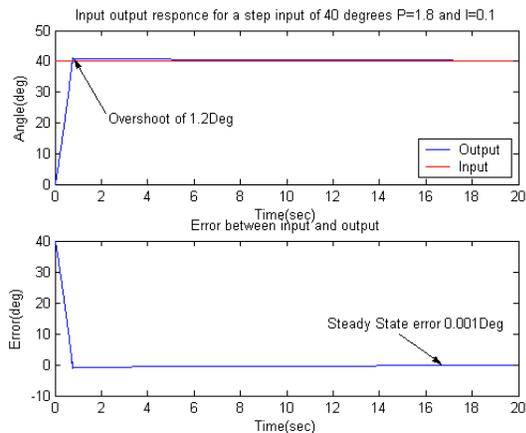
**Fig. 7. Input output plot for P=1.8 and I=0.1**
