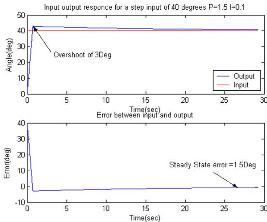
Fig. 12. Input output plot for P=1.5 I=0.1
