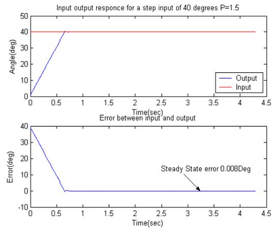
**Fig. 9. Input output plot for P=1.5**
