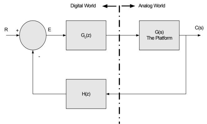
Fig. 2. Elementary Feedback Control System
