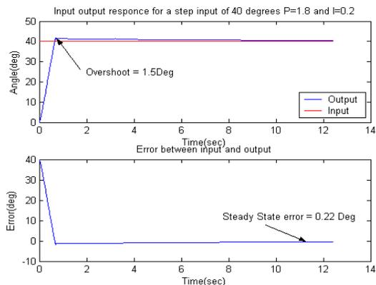
**Fig. 8. Input output plot for P=1.8 and I=0.2**
