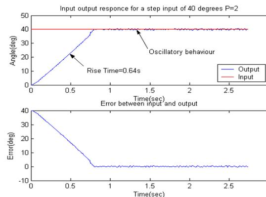
**Fig. 11. Input output plot for P=2**
