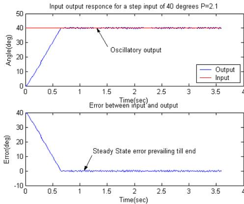
**Fig. 6. Input output plot for P=2**
