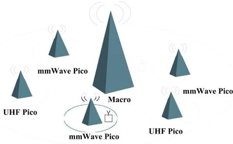
Fig. 1. System model of mmWave enabled 3-tier HetNet.
