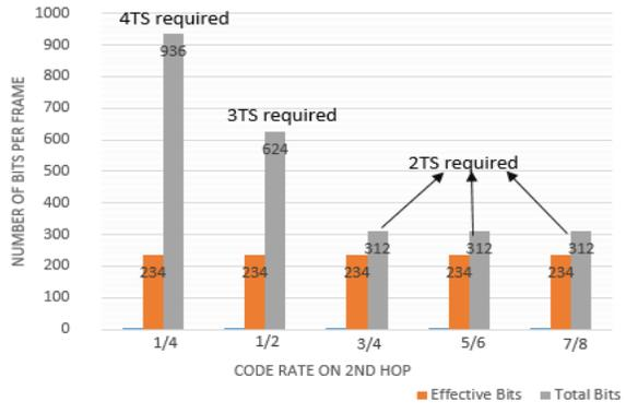
Fig. 3. Two-hop system with an LDPC code, fixed code rate on first hop =  $3/4$  and a variable rate on second hop
