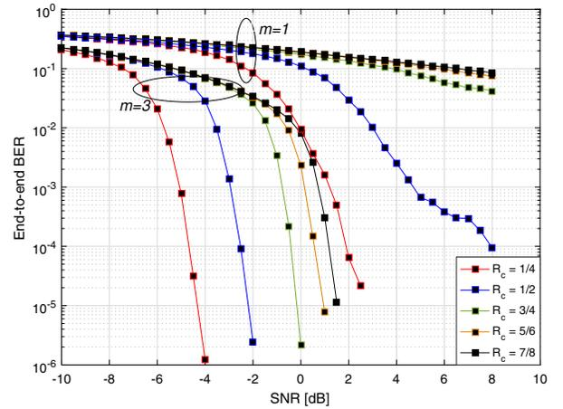
Fig. 1. BER performance at the destination node for LDPC code length  $N = 312$ , 4-QAM,  $m=1$ ,  $m=3$
