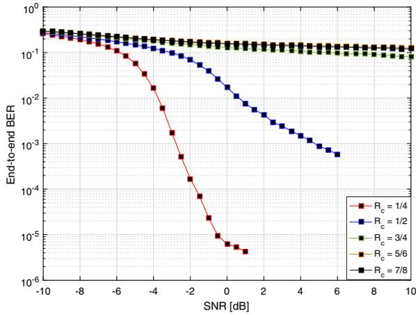
Fig. 2. BER performance at the destination node for LDPC code length  $N = 312$ , 16-QAM,  $m=3$
