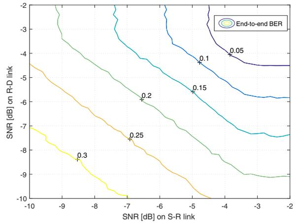
Fig. 4. A contour of SNR on two-hop relaying system
