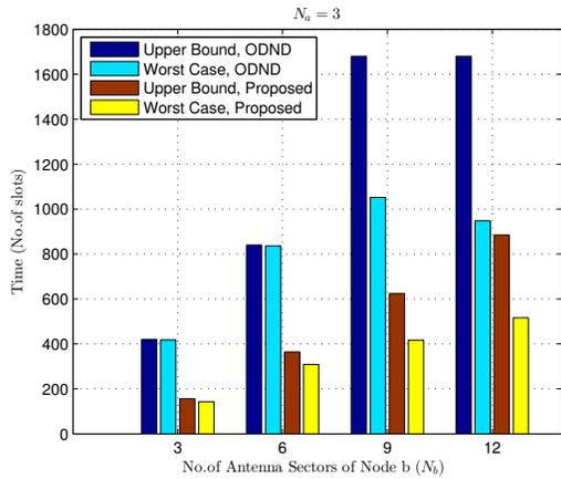
Fig. 6: Discovery delay comparison between proposed algorithm and ODND at  $N_a = 3$ .
