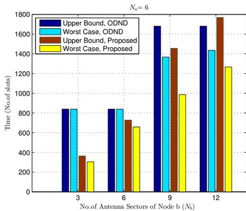
Fig. 7: Discovery delay comparison between proposed algorithm and ODND at  $N_a = 6$ .
