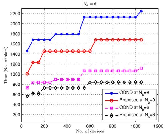
Fig. 5: Discovery delay upper bound comparison between ODND and proposed algorithm.
