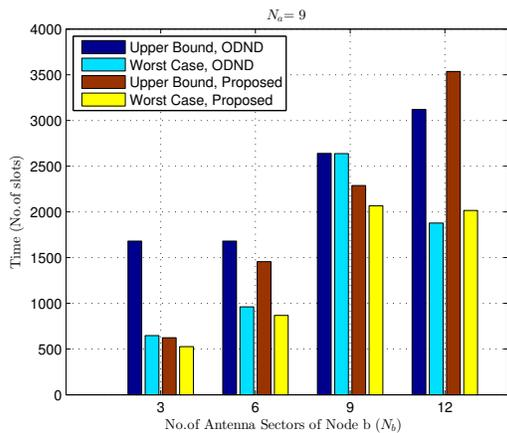
Fig. 8: Discovery delay comparison between proposed algorithm and ODND at  $N_a = 9$ .
