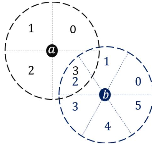
Fig. 1: Antenna configuration of two nodes  $a$  and  $b$ . Node  $a$  has 4 antenna sectors and node  $b$  has 6 antenna sectors ( $N_a = 4$ ,  $N_b = 6$ ).
