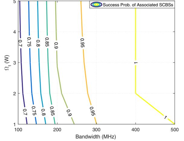
Fig. 2. The contour plot of the success probability of associated SCBSs against  $\Omega_t$  and  $W$  for the proposed approach with constraints  $R_B = 1.7$  Gbps, and  $L = 11$  averaged over 1000 iterations. (Approach 2)
