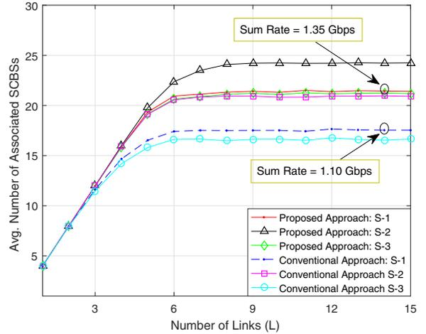
Fig. 3. Number of Links vs Average Associated SCBSs with constraints  $R_B = 1.4$  Gbps,  $\Omega_t = 1.3$  W, and  $W = 200$  MHz averaged over 1000 iterations for all scenarios.
