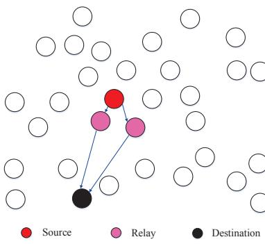
Fig. 2: Transmission to a distant node.
