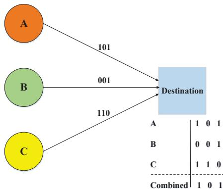
Fig. 4: Post-detection combining.
