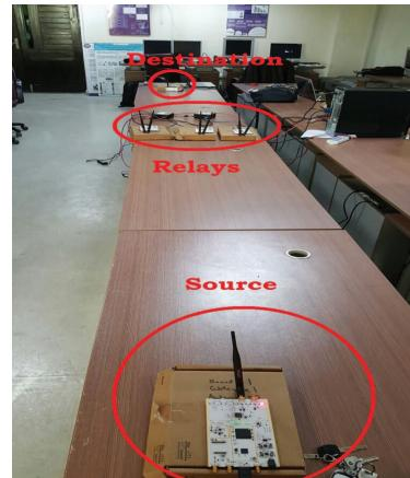
Fig. 5: The experimental setup.
