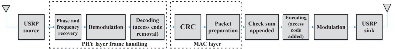
Fig. 3: Transceiver design.
