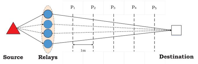
Fig. 6: Topology for determining optimum node placement.
