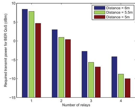
Fig. 11: Range comparison between SISO and CT networks for obtaining a QoS BER of  $10^{-4}$ .
