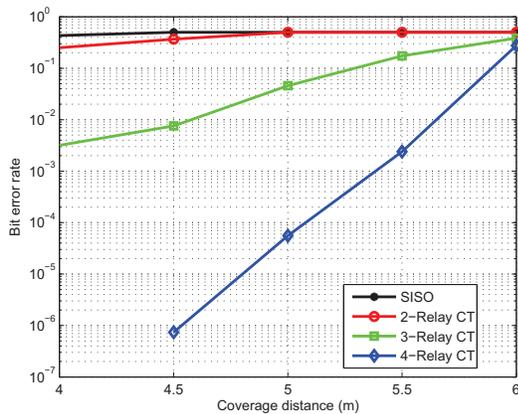
Fig. 8: BER versus source-destination distance plot, with a source power of -10 dBm
