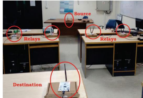
Fig. 5: Test setup for cooperative network.
