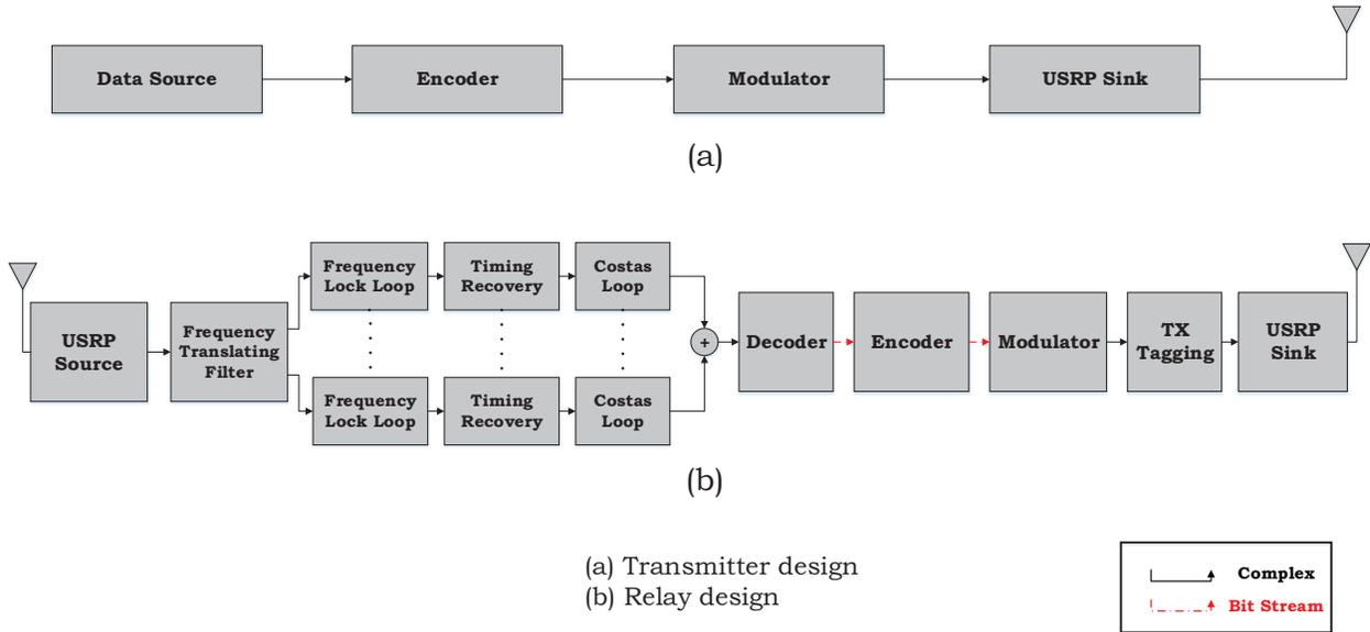
Fig. 2: Transceiver Design
