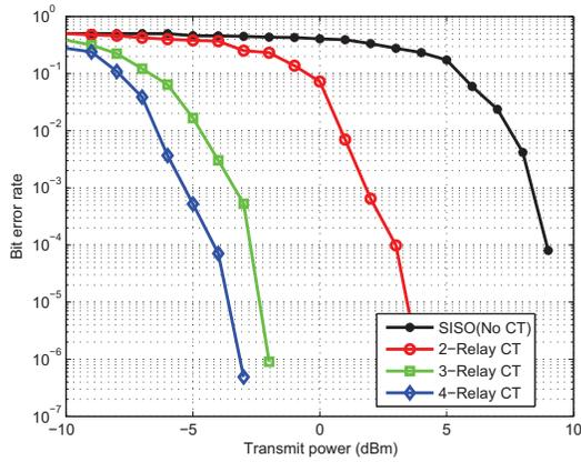
Fig. 7: BER results for SISO and CT topologies at a source-destination distance of 6m
