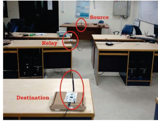
Fig. 4: Test setup for SISO link.
