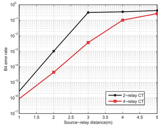
Fig. 10: BER versus source-relay distance plot.
